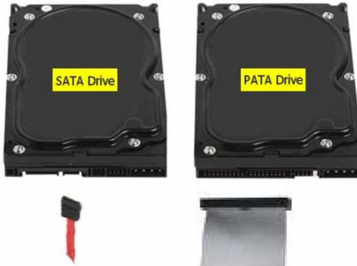
It is important that the replacement PATA drive has the Master/slave jumpers configured as per the original drive. The SATA drive does not have any jumpers but it is important that it is connected to the correct cable.
